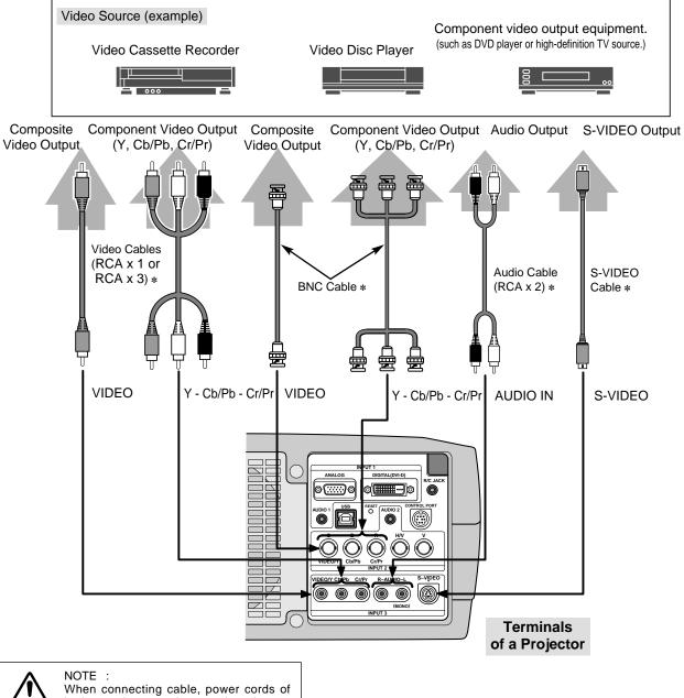
both a projector and external equipment should be disconnected from AC outlet.
